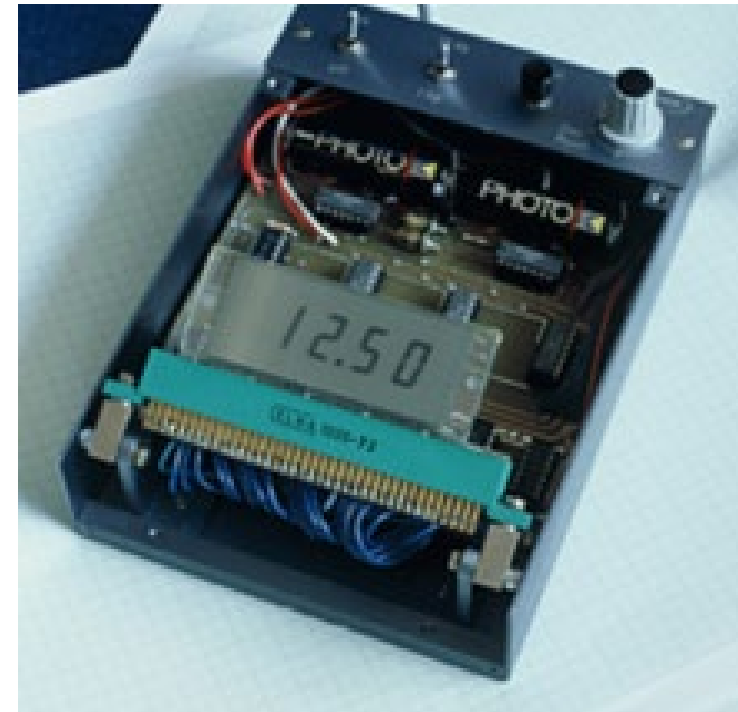
First digit prototype TNLCD made in 1971 at Hoffmann-La Roche
